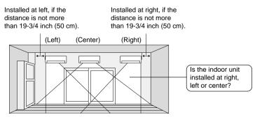
**NOTE:** If the indoor unit is installed more than 19-3/4 inch (50 cm) away from the side walls, cabinets or other nearby objects, set the slide switch to the "center" position.
